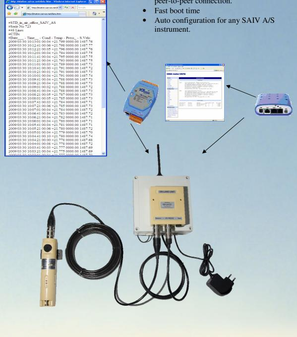
The CU801 is a unit for governing data acquisition on measuring stations/buoys in the field. It is based on dynamic web pages that are continuously updated by data from a connected instrument/sensor. The CU801 consists of an embedded web server and network router that communicates on the global GSM network with possibility of using GPRS/EDGE/3G for faster communication.
