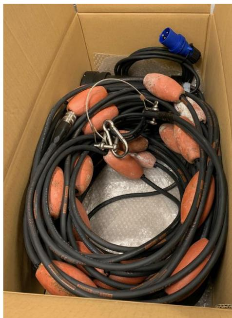
The cable must also have float devices to ensure that the cable stays floating, a cable that sinks can easily be stuck in the bottom/anchor or other underwater units. Do not use the cable more than necessary in Norway middle December to end of January.
