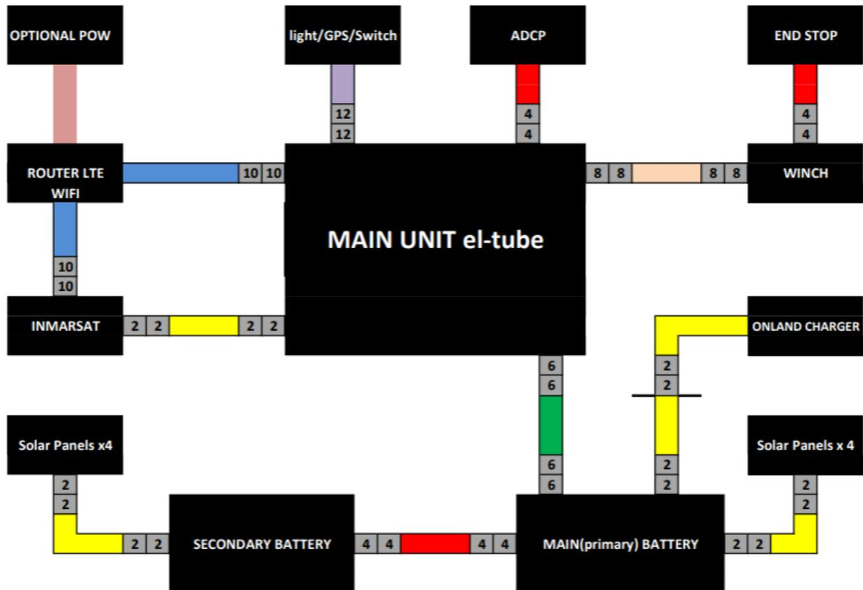
The diagram shows all units in the APB5 system and the cables between the units. The diagram also show how many pins each plug have. The ones without numbers has only pigtail.
