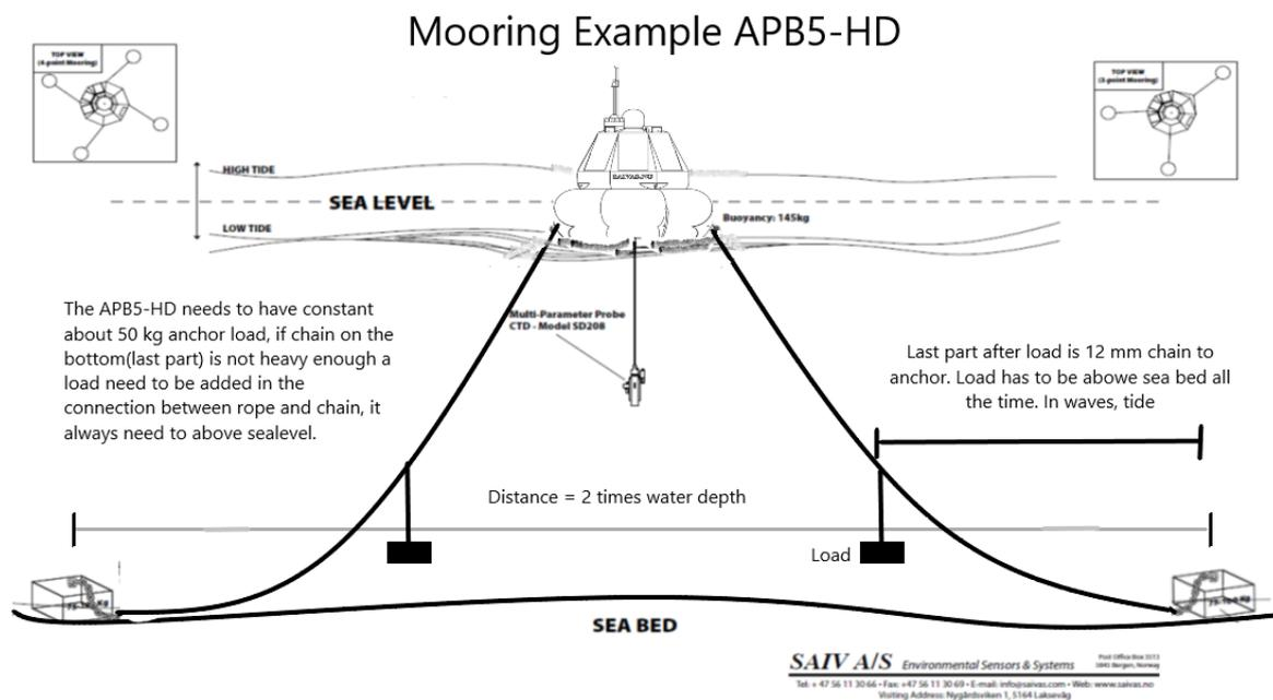
Again this mooring example is a suggestion and not a rule for all location. Therefore a local mooring company should be in charge. Things to consider: The sea floor must be checked, that it is plane. Tide, current and wave height must be in the planning.
