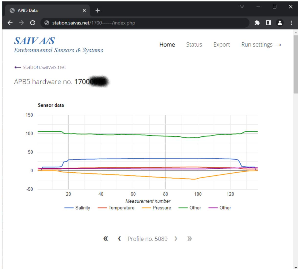
Further down on the page there is information about the profile settings, Instrument and sensors, various battery voltage and temperatures data from different units. If optional weather station w/GPS and ADCP is active their data will also be present with values if not they will be marked N/A. (Not Applicable/Available). Manufacturer information will be in the very end of the page.
