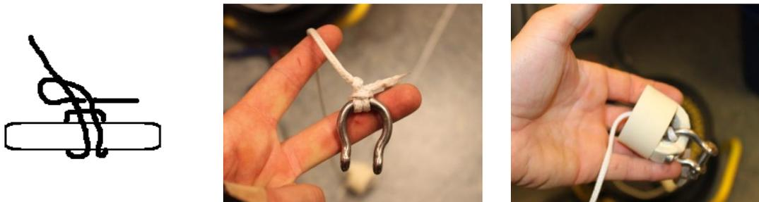
Figur 7- A clove hitch is used to fasten the CTD to the winch rope.
