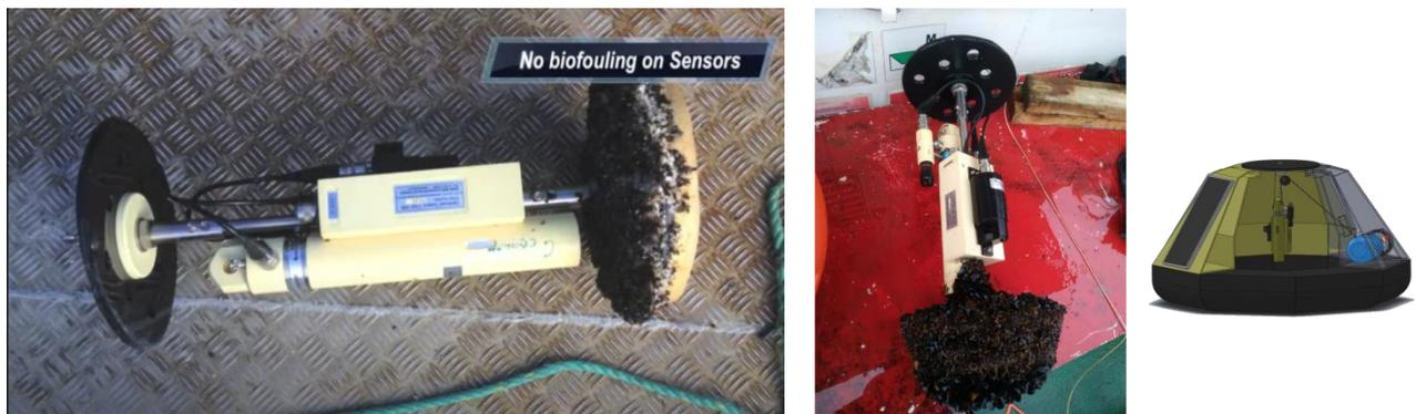
The instrument SD208 is a CTD (Conductivity Temperature Depth) with multi-parameter functionality with sensors like Oxygen, Turbidity, fluorescence and photosynthetic light sensor (PAR). The instrument is equipped with a short-range radio giving the option for cable free profiling for depth down to optional 150 meters. A wire strong Dyneema type rope 3-4 mm is proved for many years to be reliable for profiling.
