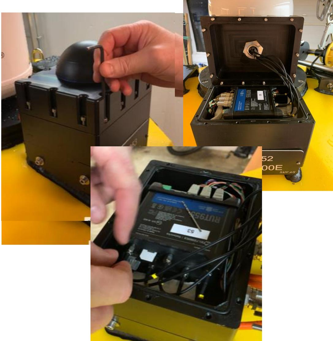
Use a 2 mm pin (like a drill or similar) to press the SIM eject button so that the SIM slot slide-out. Then change the SIM.
