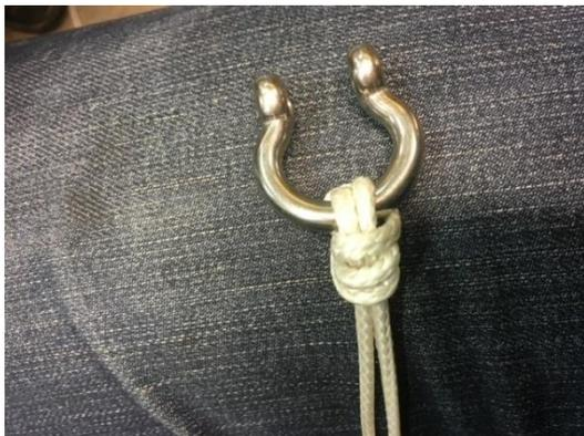
4. Three both rope ends through the end-stop. Then cut.
