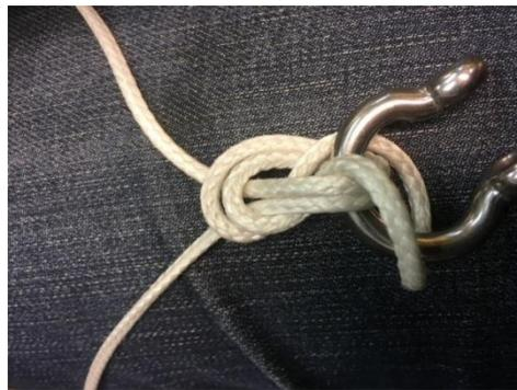
2. Then tighten in, do this in step, a lite water on the rope help.
