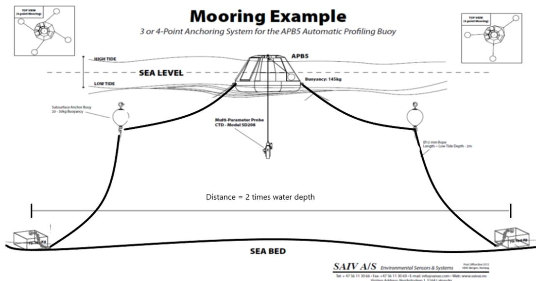
Bottom/seafloor, there should be 4 anchors with 12 mm chain connect directly and 12-14 mm rope to the APB5 or support-buoy, This is a common way to do the mooring. Anchors can be anchor rings or concrete blocks. Anchor rings can be lighter 40-70 kg. A concrete block must be heavier 100-200 kg. Weight of anchors is depended on placement of the APB5.
