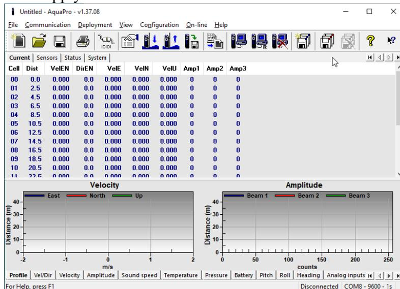
Under menu deployment, is possible to make a deployment plan. This plan will then need to be downloaded to the ADCP by update button.
