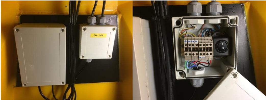
Figur 6-Power switch box inside the buoy.
