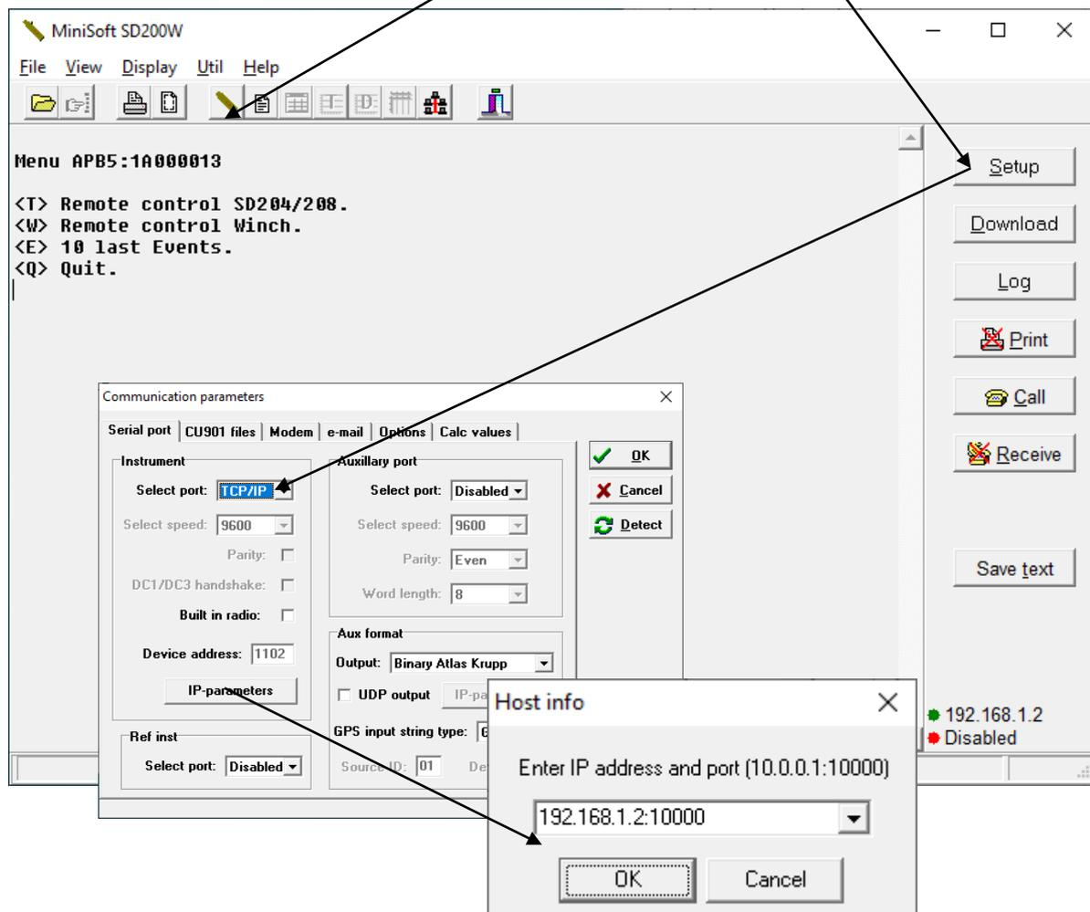
Use the menu to navigate. NB: If no selections are made APB5 will timeout after 2 minutes and close connection.
