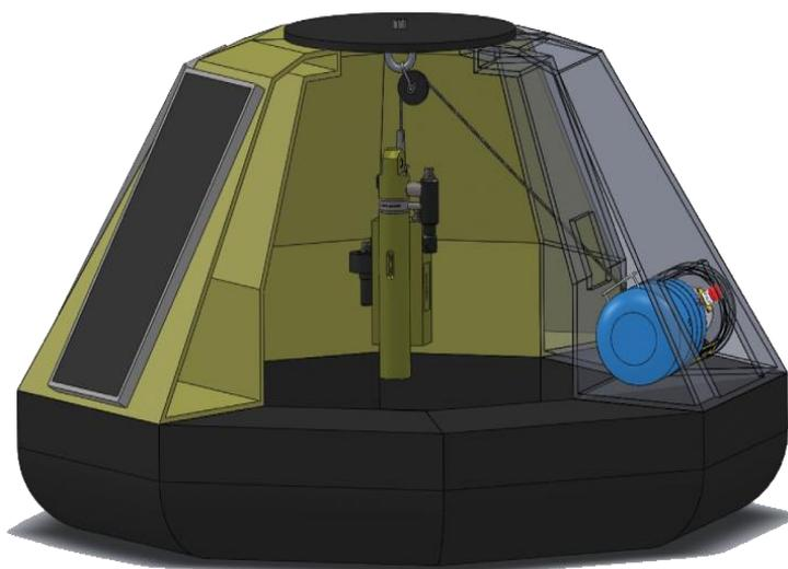
Figur 2- Cross section view of APB5 showing CTD in OWAS position.
