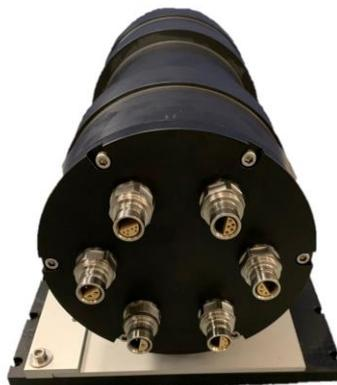
*Figur 13- Main controller/Unit el-tube w/6 different pins number.*
