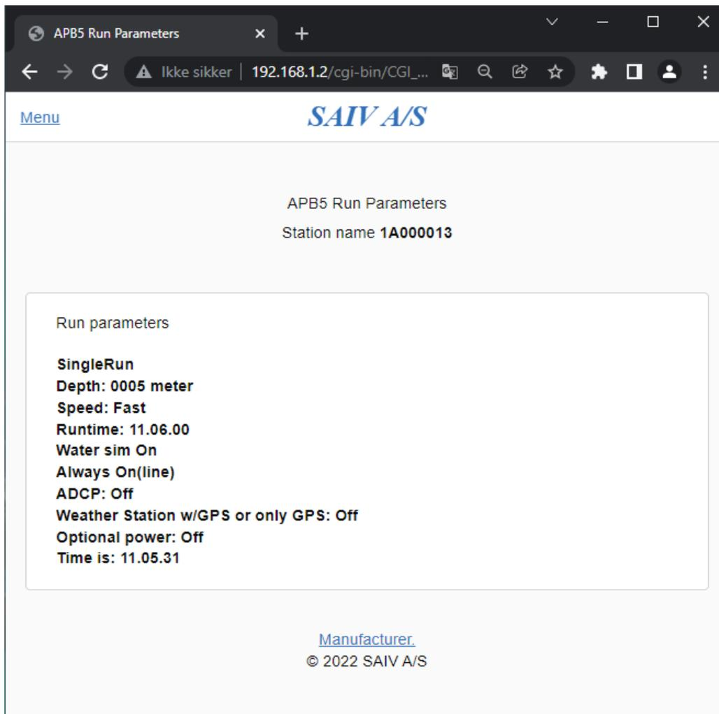
From the run parameter the water sim is on in this specific run case. This is than a land test and user must prepare to help instrument after it has rested in the climate zone for 30 seconds. This has been explained in start of this manual under “first time start up and land test” point 7.
