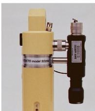
First plug in the sensor and tighten the sleeve nut completely. The sensor is now correctly connected and the securing screw can be installed. This screw has an O-ring under the head and should only be tightened lightly to allow some flexibility.
