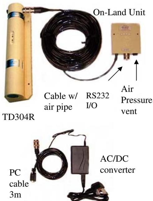
The figure to the left shows the TD304R with On-Land Unit. The On-Land Unit provides connector for direct data communication and ventilation to air pressure.
